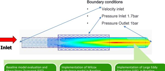
Shear Stress Transport (SST) turbulence model implementation
