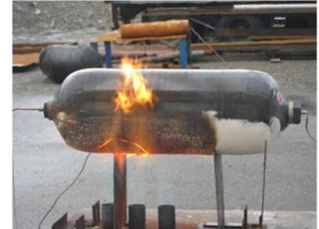
Source: Powertech Localized Fire Protection Assessment for Vehicle Compressed Hydrogen Containers, 7/23/09
