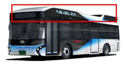
• If the CHSS is located at the lower position, there is the probability of hydrogen leakage in case of side impact crash
