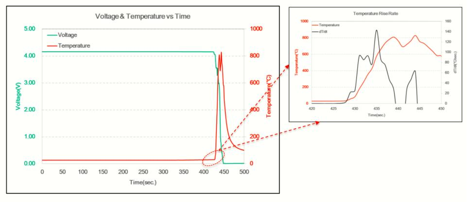
The temperature rise rate was >>1°C/s, so the cell had thermal runaway.
