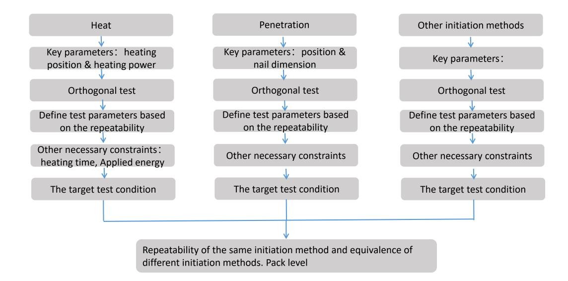
• For heating: mainly investigates two key parameters of heating position and heating power.
