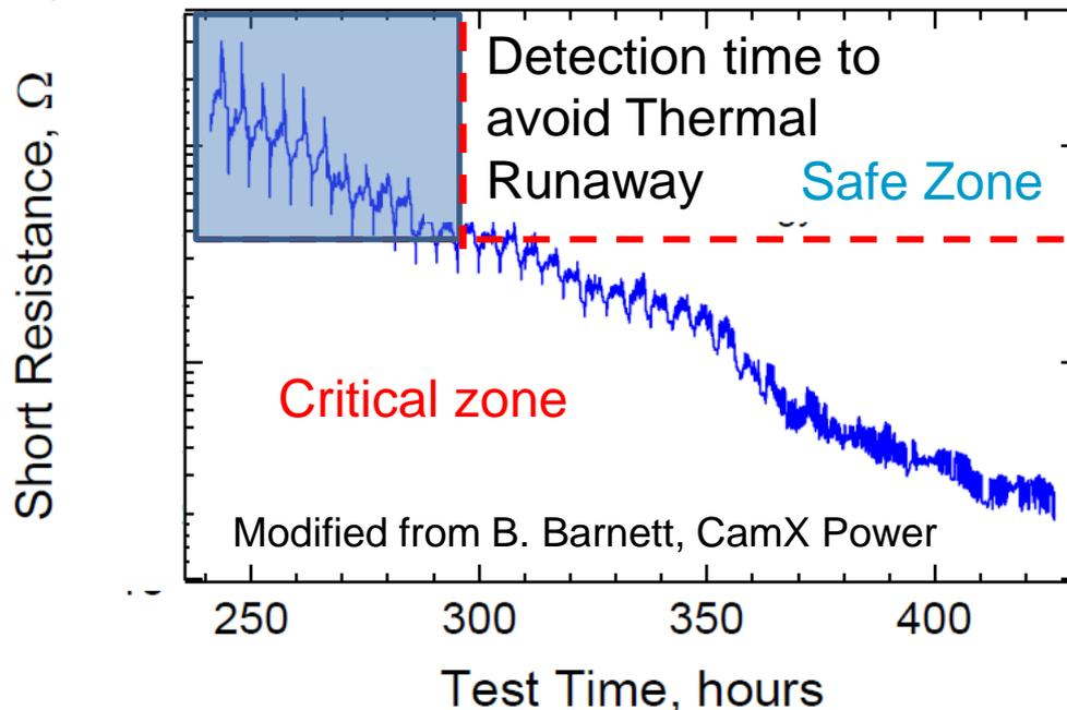
The ISC-induced Joule heating will not develop into thermal runaway until the ISC resistance decreases to a low level, which varies for every cell/chemistry/design/etc etc.
