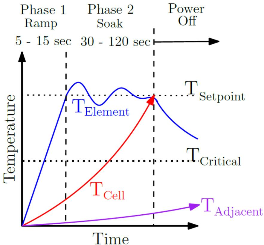
Requires  $T_{Setpoint}$  and Ramp/Soak time definitions within test method.
