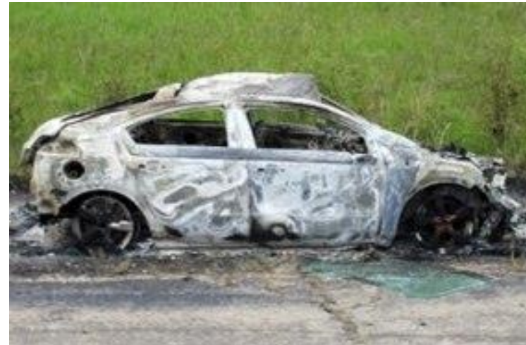
Pole tested Chevrolet Volt after the fire at MGA reported on June 6, 2011.
