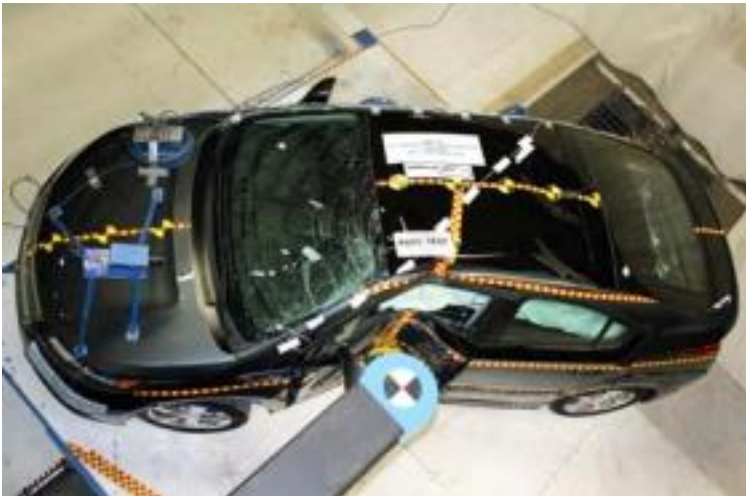
Chevrolet Volt after being subjected to the NCAP pole test on May 12, 2011 at the MGA test facility.
