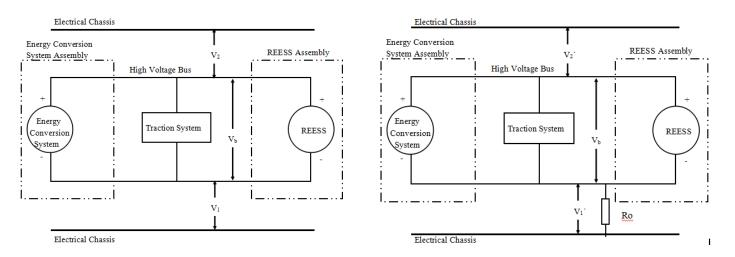
1st: Run the circuit, V<sub>b</sub> is higher than nominal voltage;
