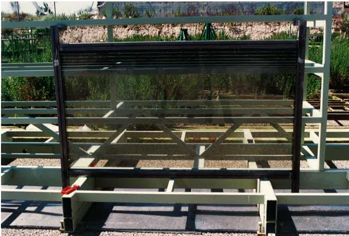
Figure 24: Frame structure of windows. Glass breaking tests.
