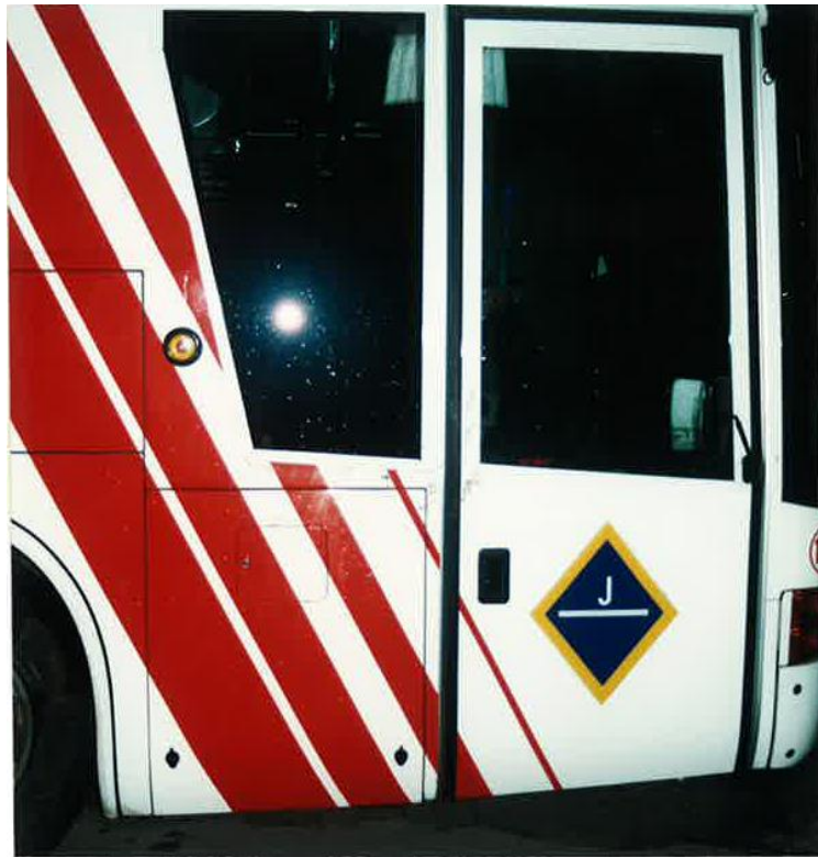
Figure 9: External control location on the front door (vehicle identical to the accident).
