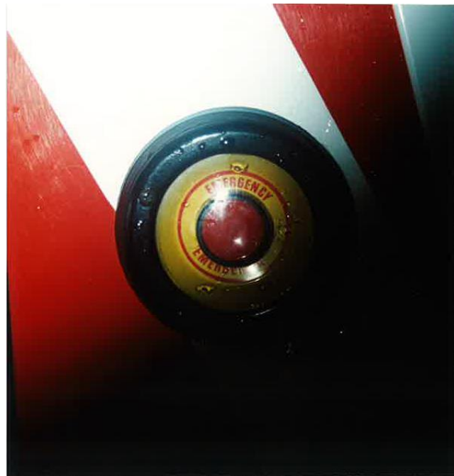
Figure 10: External control detail on the front door (vehicle identical to the accident).
