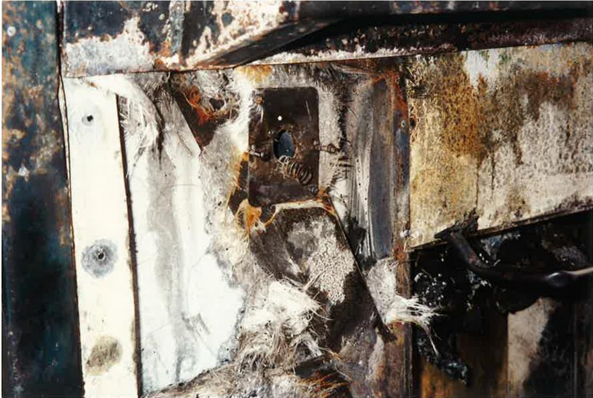
Figure 19: Detail of interior control in rear door (accident vehicle).
