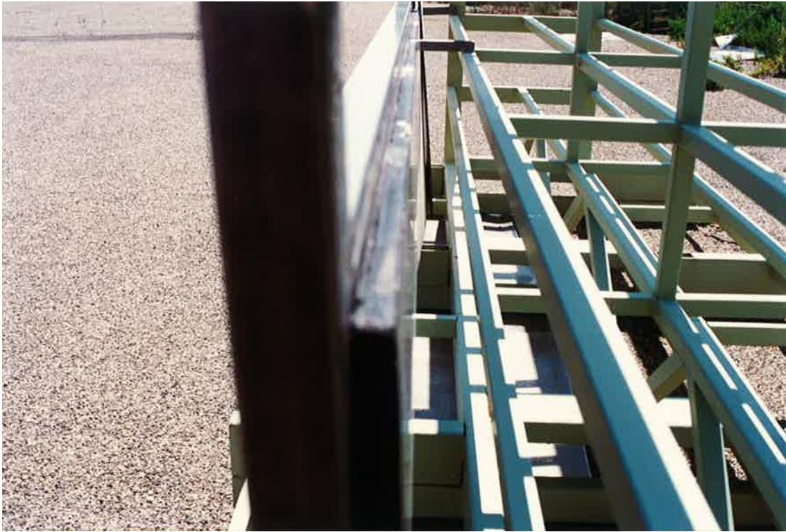
Figure 23: Adhesive fixing glass windows to the frame. Glass breaking tests.
