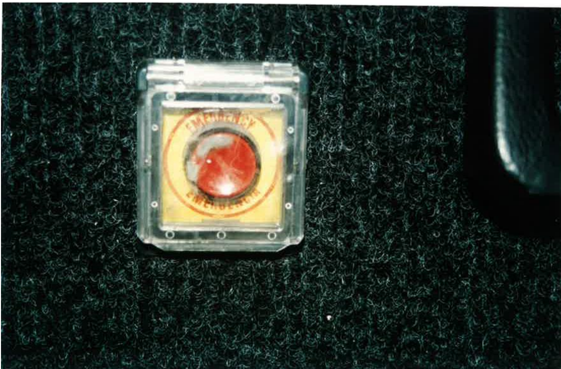
Figure 18: Detail of interior control in rear door (vehicle identical to the collided one).
