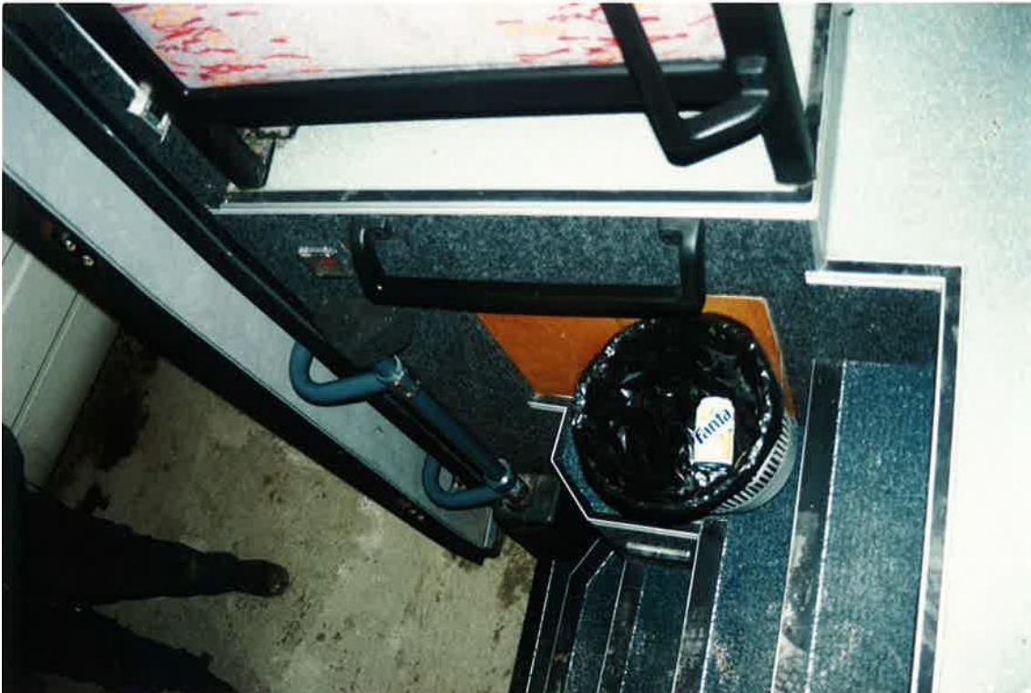
Figure 17: Location of internal control in the rear door (vehicle identical to the collided one).
