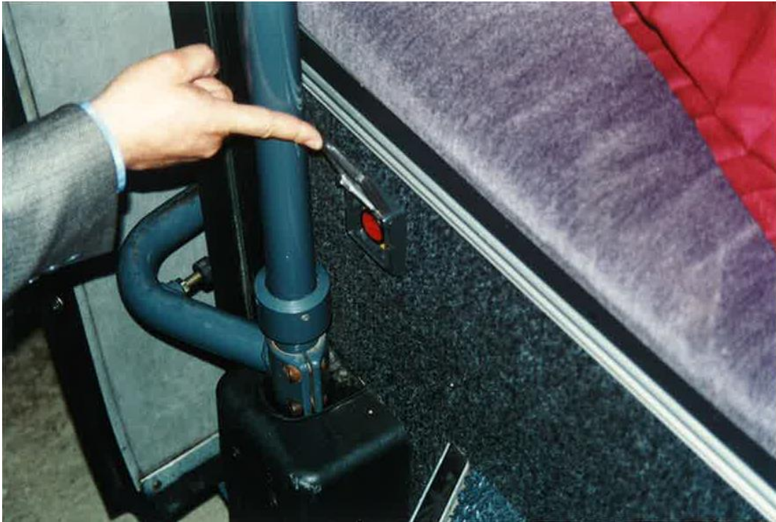
Figure 13: Location of internal control in front door (vehicle identical to the collided one).
