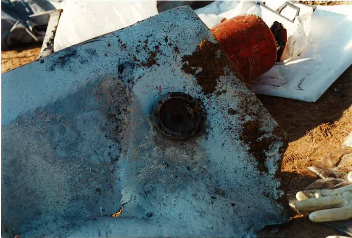
Figure 16: Detail of external control in rear door (accident vehicle).
