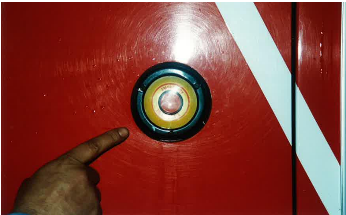
Figure 15: Detail of exterior control in the rear door (vehicle identical to the collided one).
