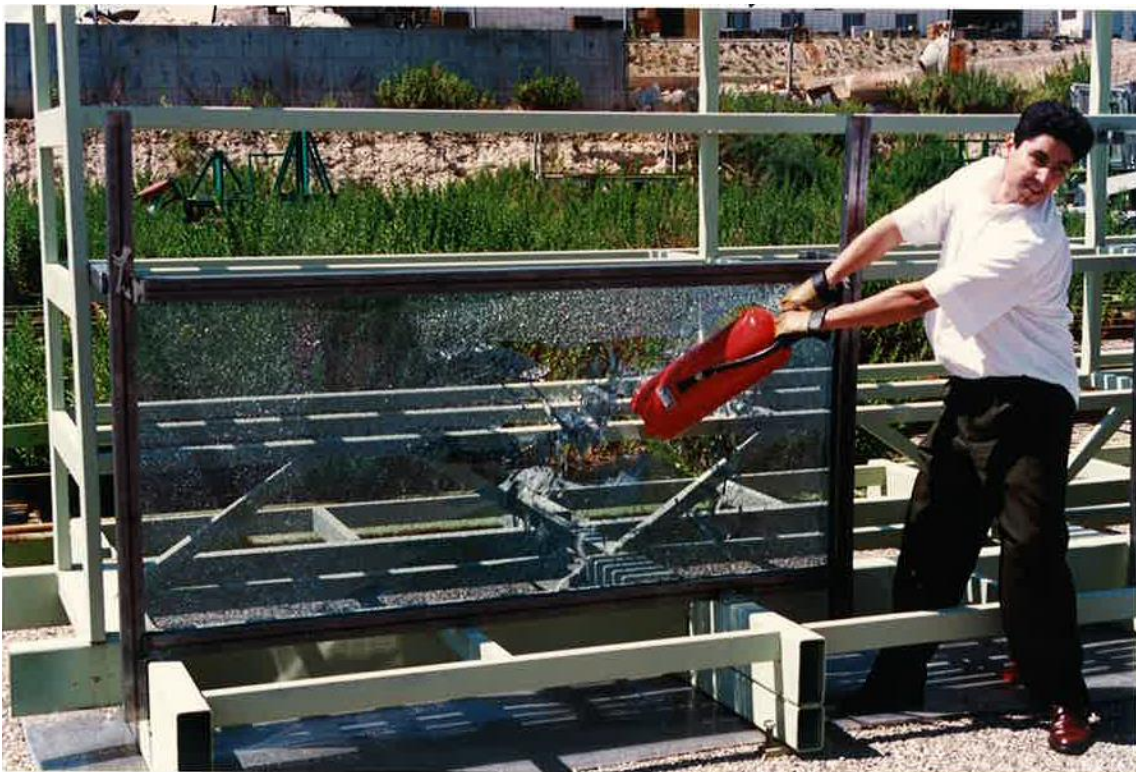
Figure 26: Simple moon break with fire extinguisher.
