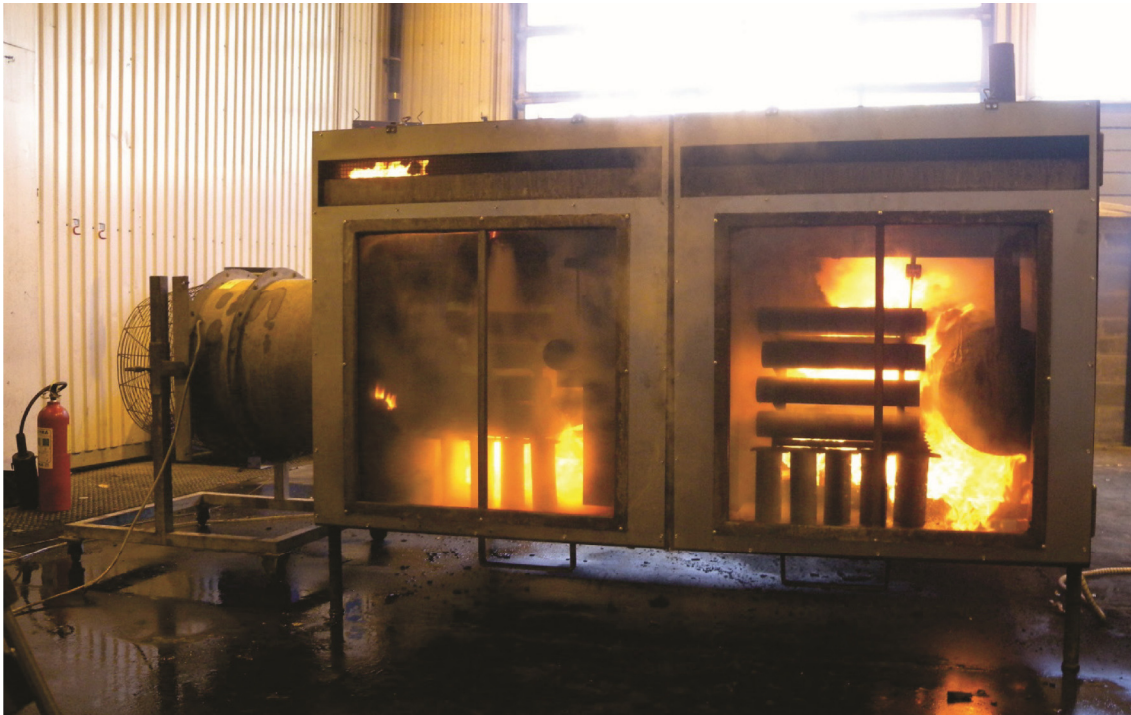
Figure 4 Fire test according to SP Method 4912. A fan is seen to the left.
