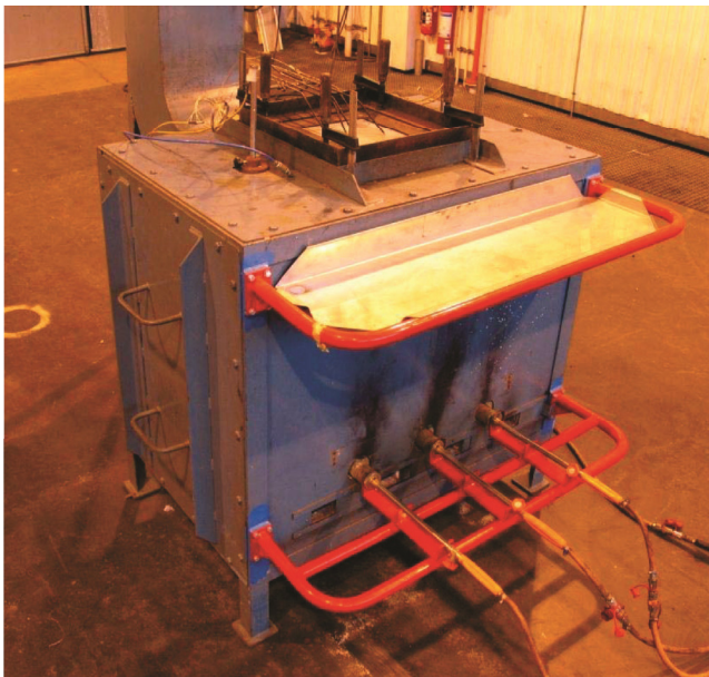
Figure 5 Furnace to assess fire resistance of partitioning as proposed by Hammarström et. al [31].
