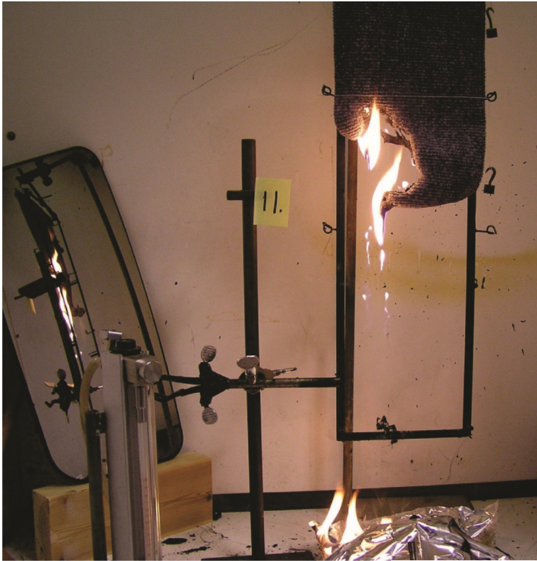
Figure 2 Test to determine the vertical burning rate according to Regulation No. 118.
