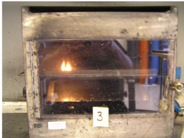
Figure 2. Test of product no. 3 according to ISO 3795.
