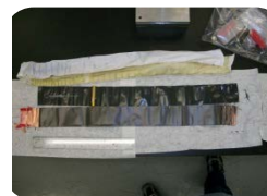
Unrolled anode, cathode, and separator
