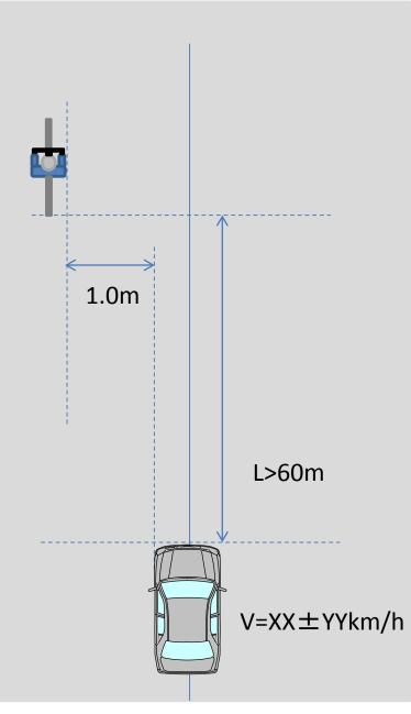
VRU Soft Target(a) So as to face in the same direction of travel as the target,(b) With a distance of 1.0 m between Vehicle under test and Target,
