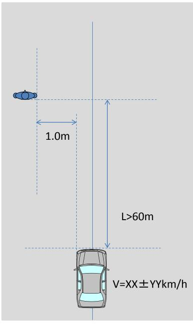
VRU Soft Target(a) So as to face in the same direction of travel as the target,(b) With a distance of 1.0 m between Vehicle under test and Target,
