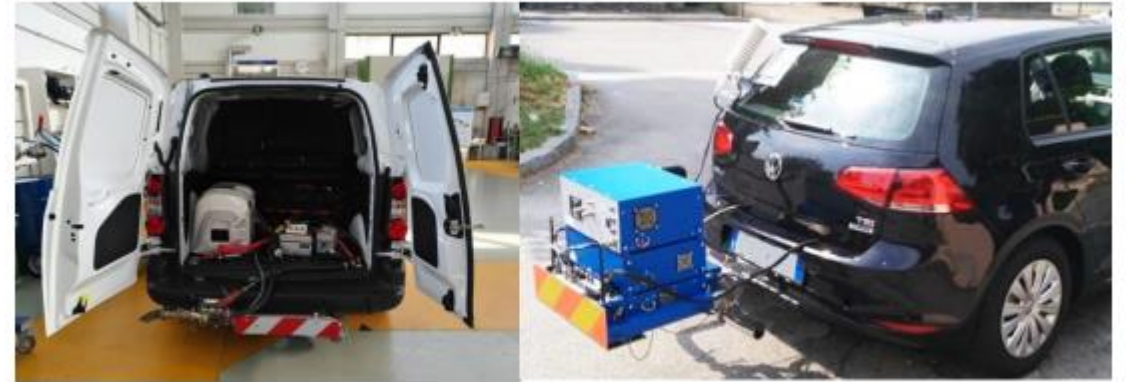
Figure 1. Installation of PEMS main units (left) inside the vehicle (right) outside the vehicle
