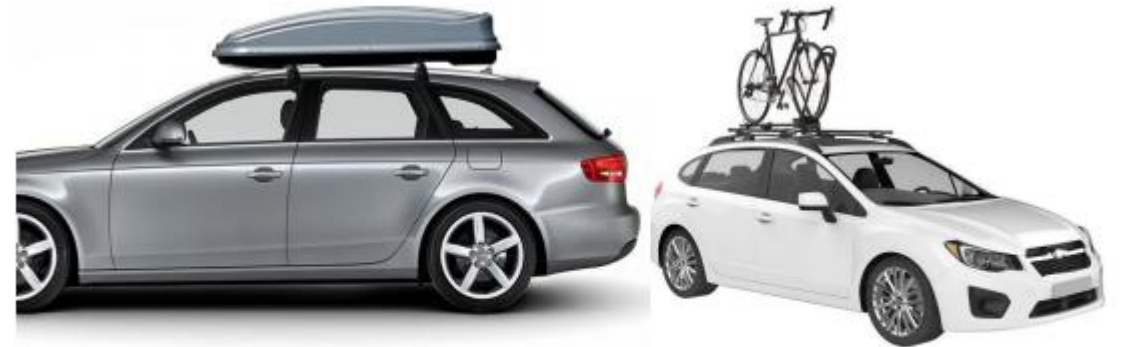
Figure 2. Vehicles equipped with a roof box (left) or loaders that modify the aerodynamic characteristics of a vehicle (right) are not eligible for RDE-TA and RDE-ISC testing.
