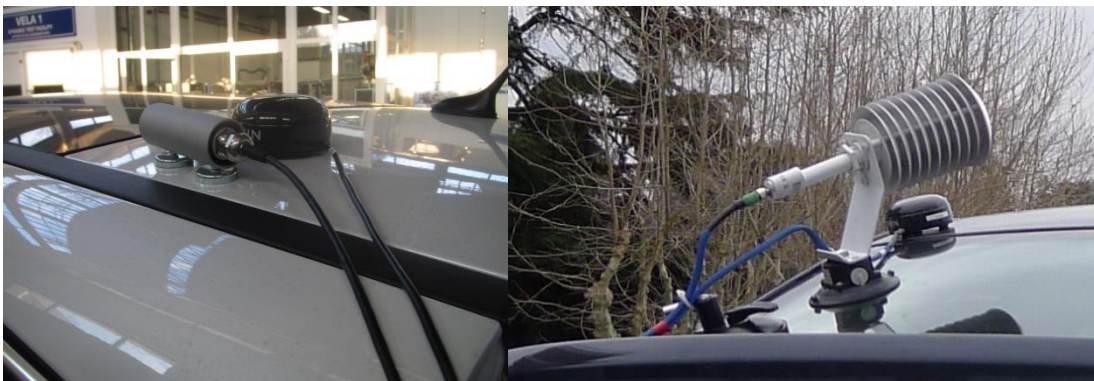
Figure 6. Installation examples for the GPS antenna and the weather station
