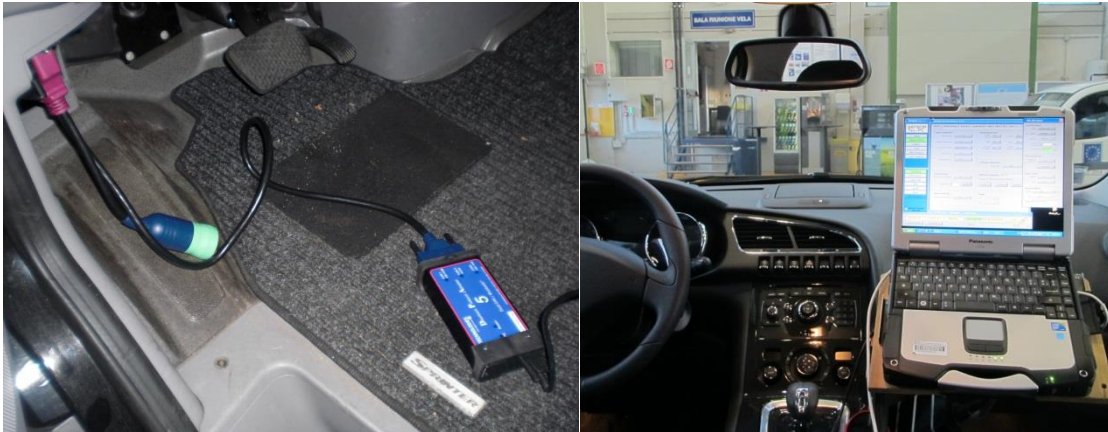
Figure 7. left) connection to the vehicle ECU, right) secure mounting of a laptop connected to the OBD reader.
