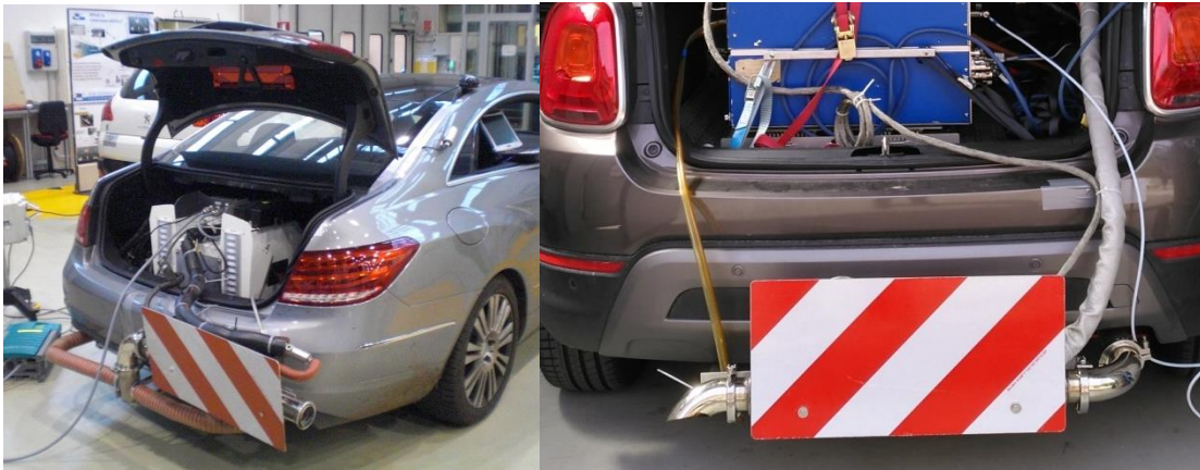
Figure 5. left) examples of EFM installation when the PEMS main unit is installed inside the vehicle; right) proper signalling of the EFM
