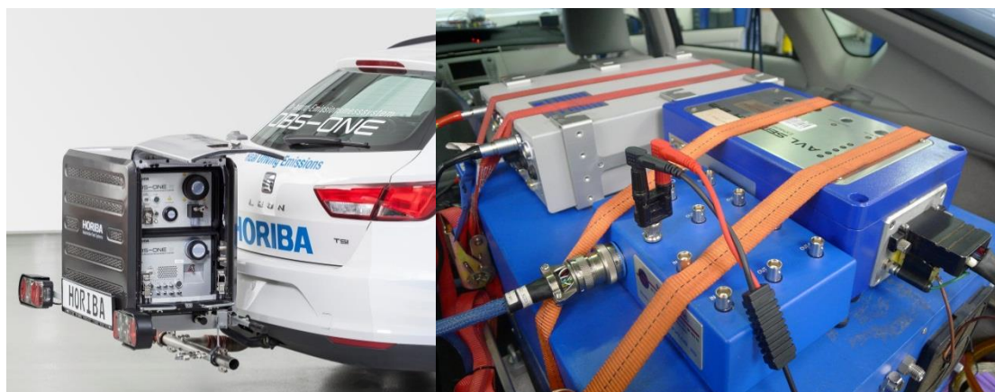
Figure 3. left) installation of PEMS main units outside the vehicle; right) securing the instruments with straps inside the vehicle
