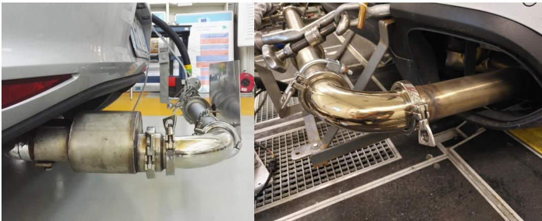
Figure 4. EFM Installation left) using a tailpipe adaptor; right) tubes and collars on a dual exhaust
