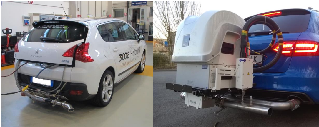
Figure 9. Routing heated probe left) from the inside of the vehicle; right) outside of the vehicle
