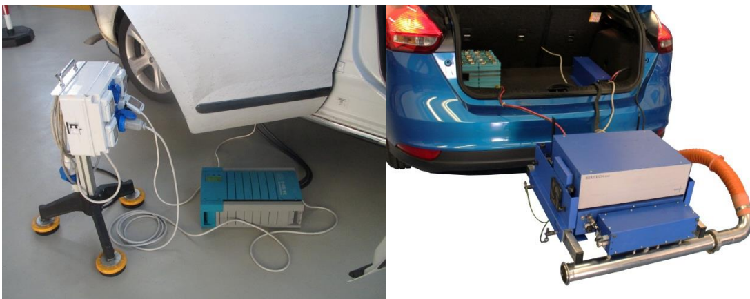
Figure 8. left) Charging of the batteries; right) batteries to operate the PEMS, located in the trunk, properly secured with straps
