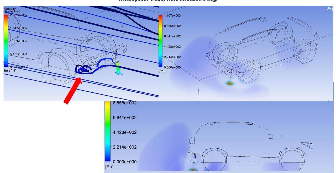
**Simulation results** Wind speed: 5 m/s; wind direction 0 deg. 3.764e+002 3.764e+002 3.614e+002 3.614e+002 3.463e+002 3.463e+002 3.312e+002 3.312e+002 3.162e+002 3.162e+002 3.011e+002 3.011e+002 [K] 3.764e+002 3.614e+002 3.463e+002 3.312e+002 3.162e+002 3.011e+002
