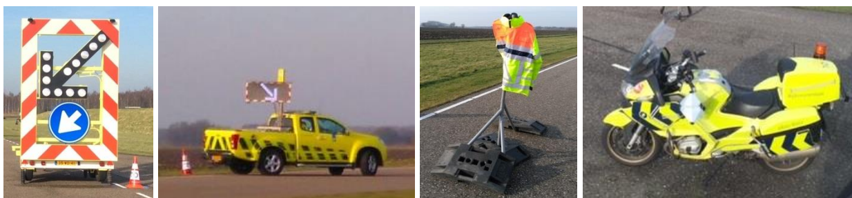
Figure 1 Traffic control measures tested: traffic arrow trailer, WIS car fend-off, WIS jacket, WIS motorcycle.
