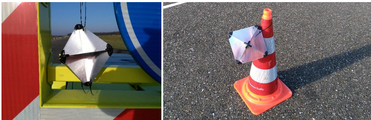
Figure 9 – Reflector attached to traffic arrow trailer (left) and to a 75 cm pylon (right).
