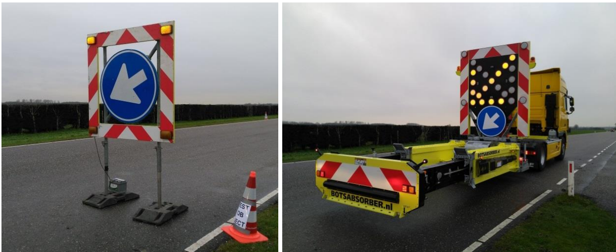
Figure 14 – Mobile road sign (left) and collision absorber (right).
