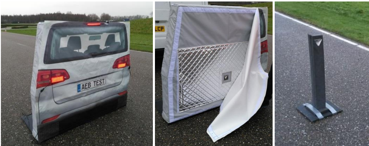
Figure 15 – Moshon Data Slab Foam Target (left and centre) and Moshon Data Delineator (right).
