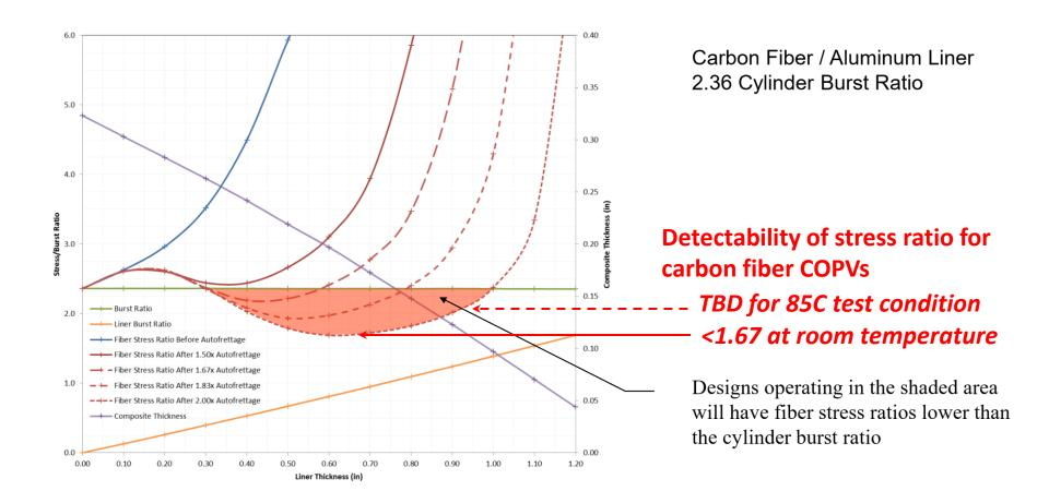
CONCLUSION: Analysis at 85C IS required to judge effectiveness of the proposed stress rupture withstand test in detecting problems.
