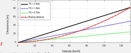
$S_{Critical-Front} = v_{ACSF} \times t_{front}$
