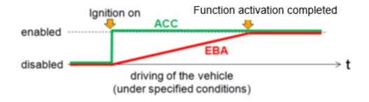
Calibration time depends on the software and is specific to the vehicle manufacturer.
