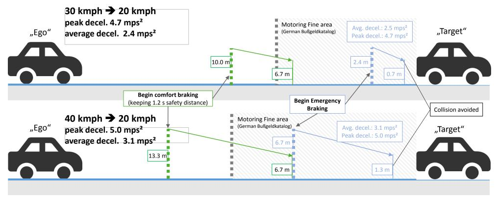
Nevertheless those AEB are **not considered convenient** – not only because of the level of the deceleration, but because of **starting and ending distance** of the braking phase itself.
