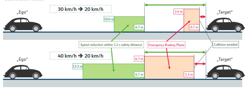
Nevertheless those AEB are not considered convenient - not only because of the level of the deceleration, but because of starting and ending distance of the braking phase itself.
