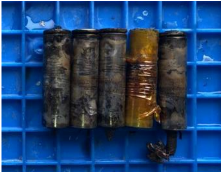
18650-2.2Ah-7.92Wh heating power: 100W
