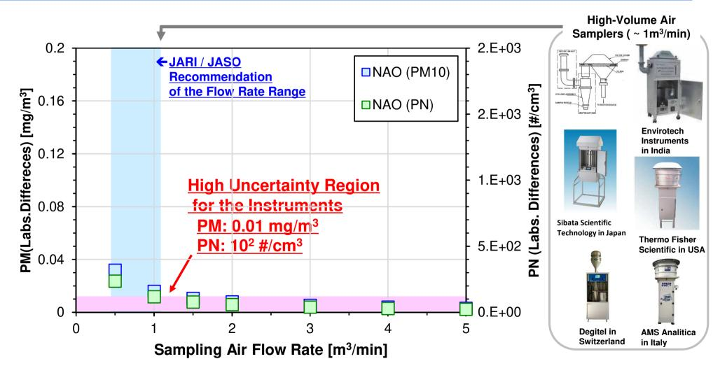
Cycle: simulated-WLTC, 30 Repeated, PM data: DustTrak II 8530 corrected by gravimetric measurement, PN data: TSI CPC 3775 (D<sub>50</sub> = 4 nm) without pretreatment
