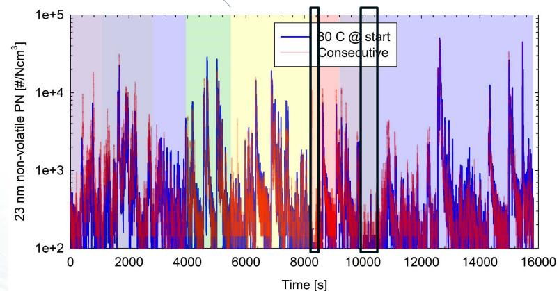
Peak concentrations exceed the single count mode  $(1-3 \times 10^4 \text{ #/Ncm}^3)$  of full flow CPCs  $\rightarrow$  dilution is required.
