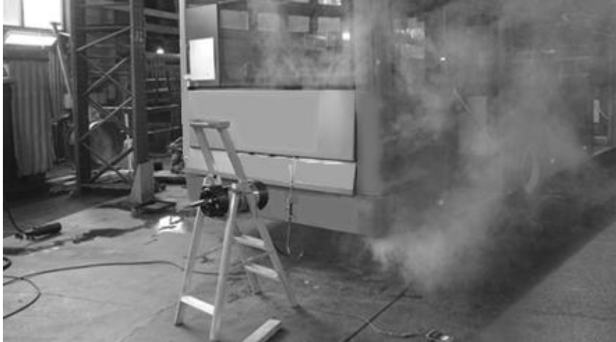
Figure 17. Diesel spray on a hotplate inside the engine compartment.
