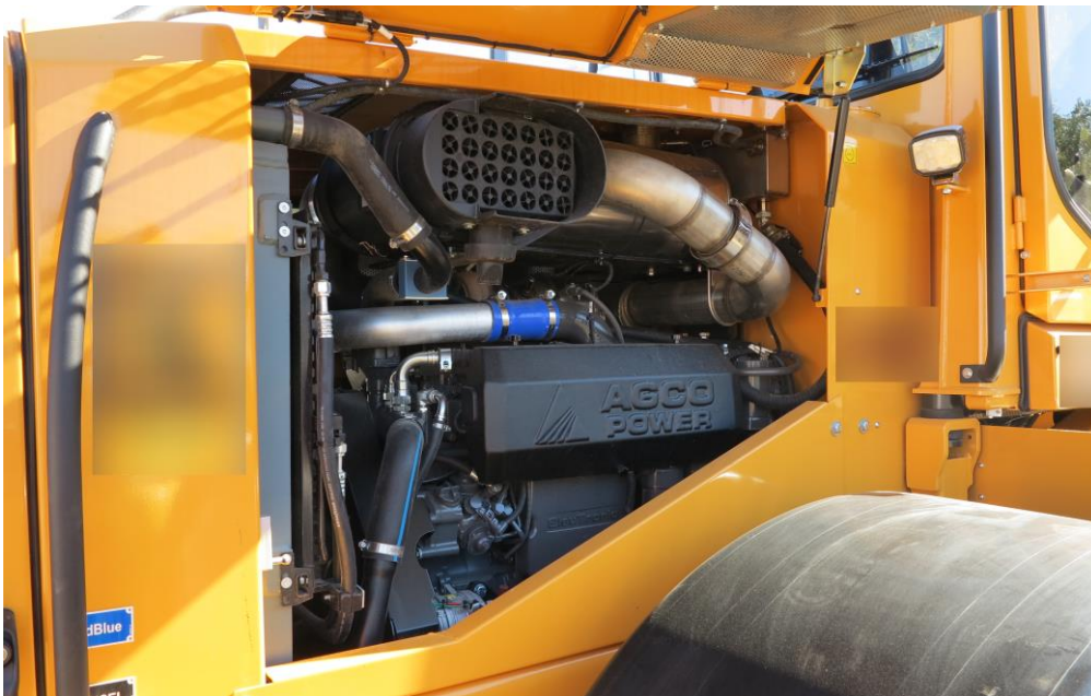
Figure 42 Engine compartment of a wheel loader, the cold side of the engine.
