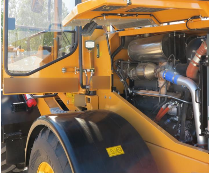
Figure 41 Engine compartment of a wheel loader, the warm side of the engine.
