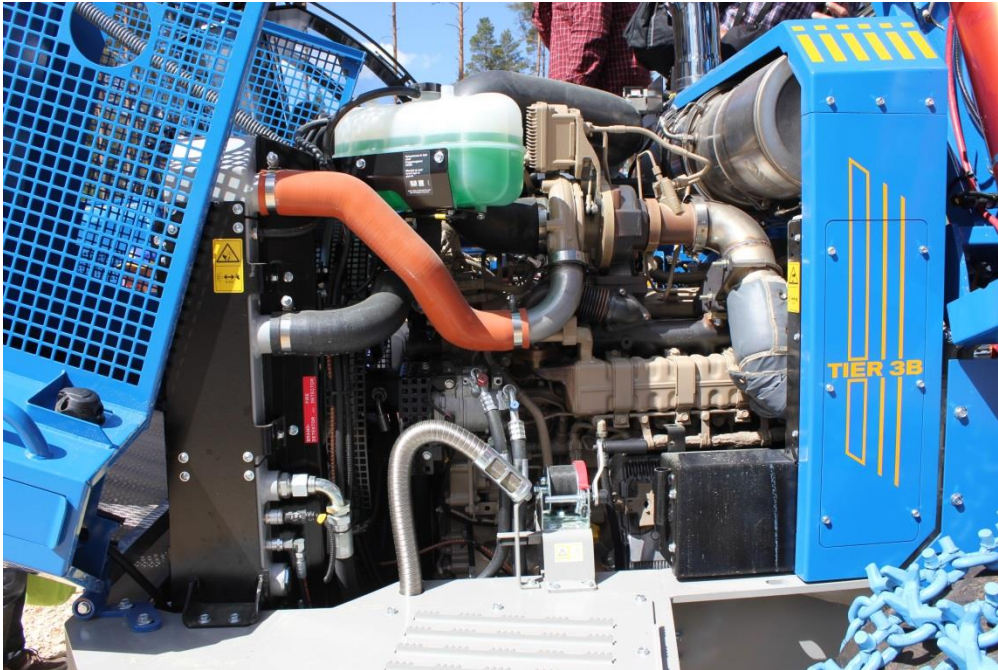
Figure 47 The warm side of the engine compartment in a forestry machine.
