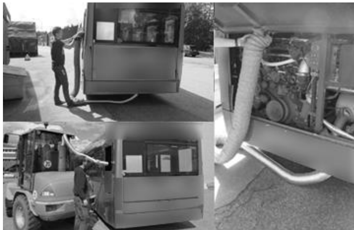
Figure 9. Exhaust is led into the engine compartment directly (right photo) or through radiator from the bus (upper left photo) or from an external truck (lower left photo).
