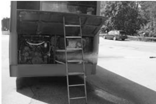
Figure 12. High pressure water spray directed towards the engine compartment.
