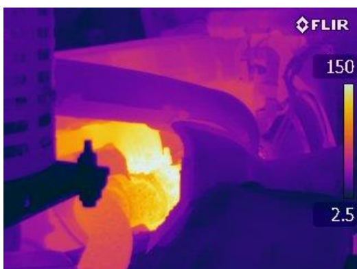
Figure 25. Thermal imaging photo of the engine block and turbocharger (similar angle as in Figure 23).
