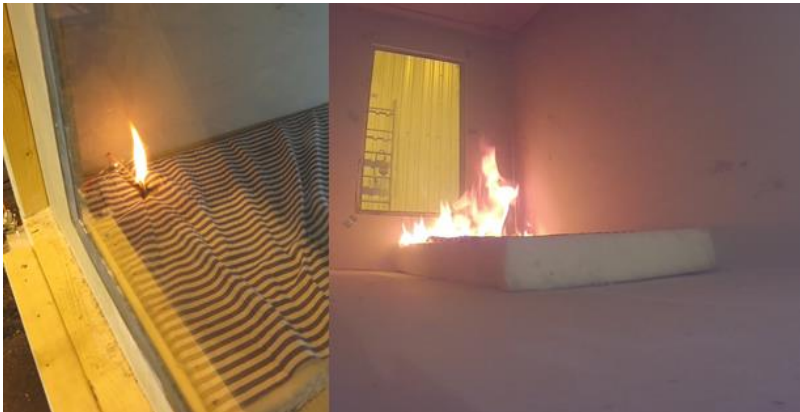
Figure 19. Mattress fire in sleeping compartment mockup.
