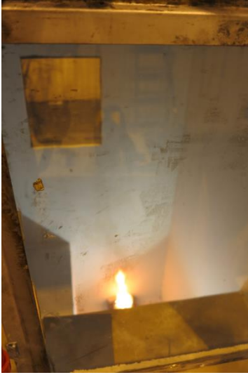
Figure 17. Heptane pool fire. Seen through the window to the left in Figure 14.
