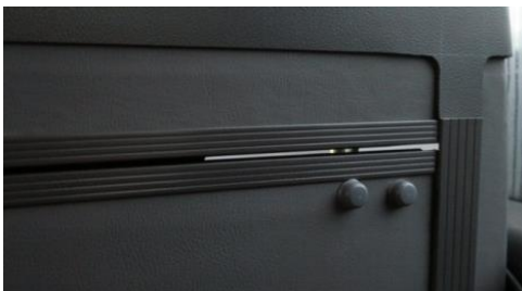
Figure 13. Example of air inlet through gaps around toilet compartment door.
