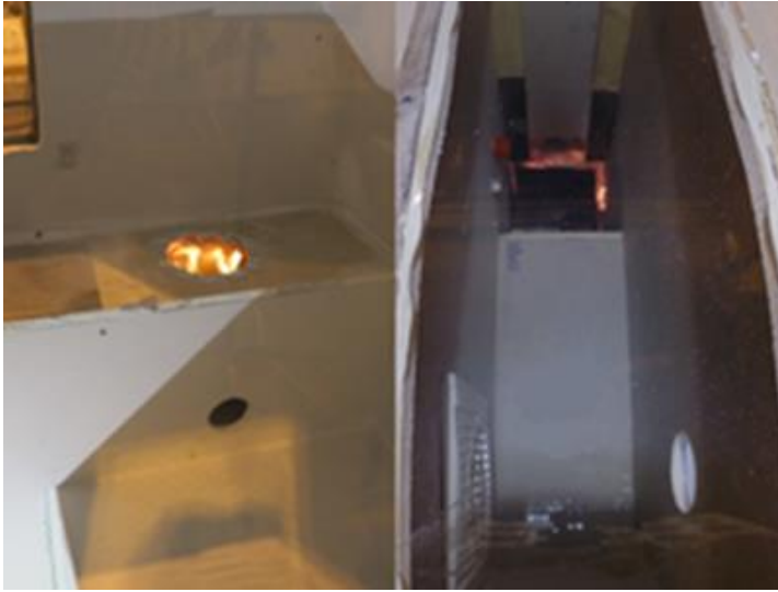
Figure 16. Trash can paper fire. Left: seen from above, Right: seen from inside the concealed space under the sink.
