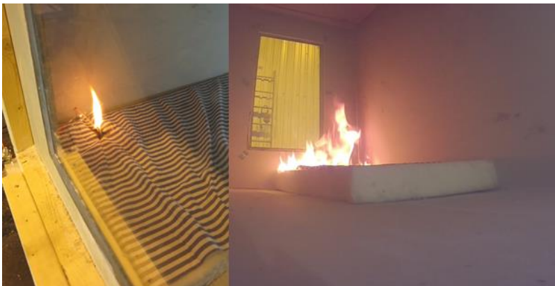
Figure 19. Mattress fire in sleeping compartment mockup.
