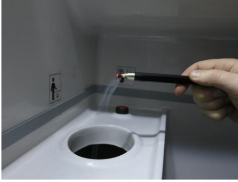
Figure 10. Smoke pen over the trash can. Smoke is drawn down towards the opening of the trash can.
