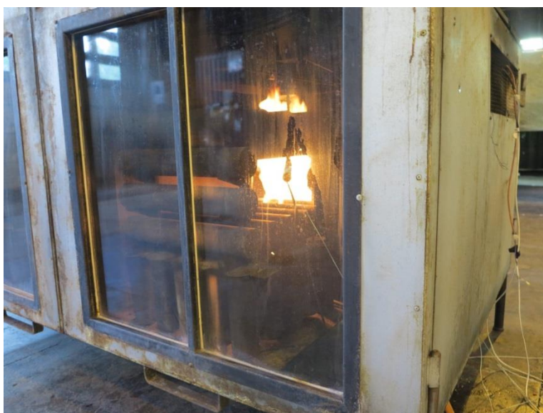
Figure 18. Heat detector fire test in an engine compartment mock-up.
