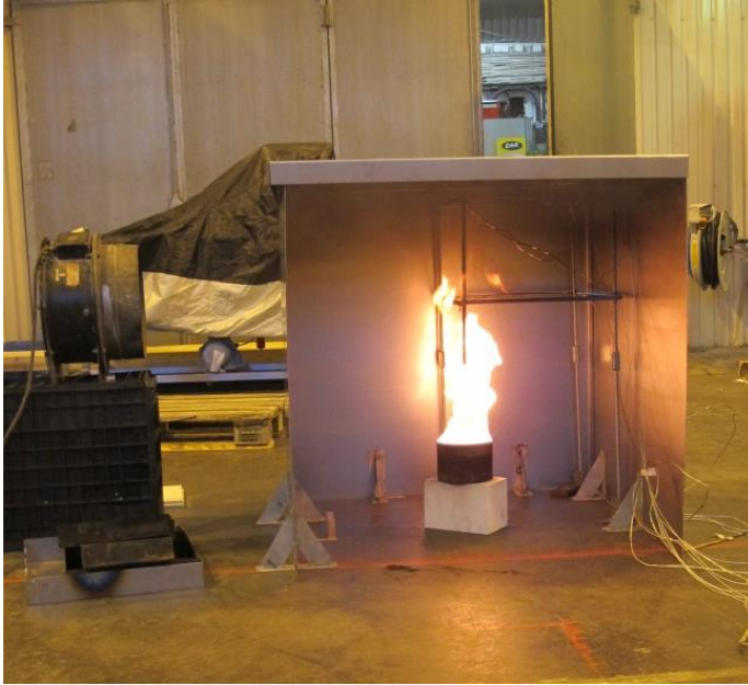
Figure 19. Heat detector fire test.
