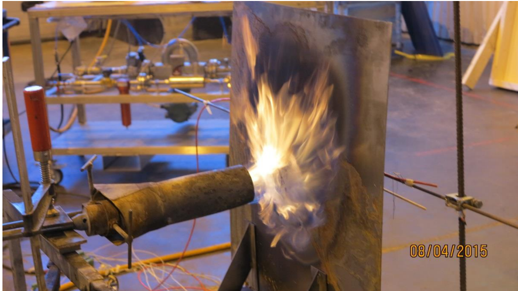
Figure 17. Metal plate heated by a LPG burner for false alarm tests.
