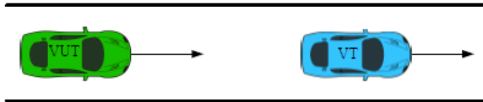
Figure 6.28 Schematic diagram of test scenario that forward vehicle applies brake
