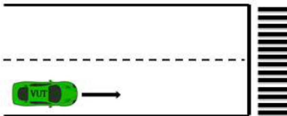
Figure 6.4 Schematic diagram of test scenario of identification and response to crosswalk lines
