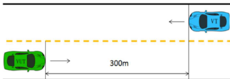
Figure 6.30 Schematic diagram of the test scenario of vehicle-to-vehicle on long straight road segment
