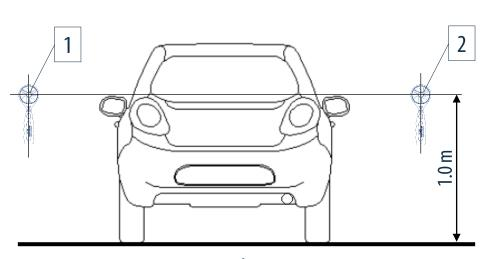
1,2 – anemometers; 3 - weather vane
