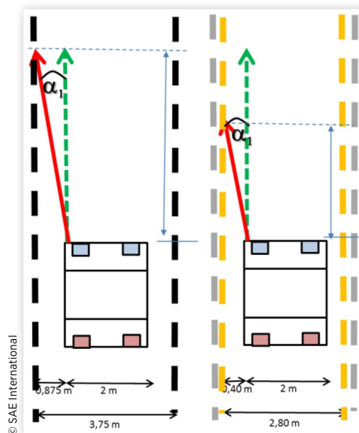
FIGURE 10 Comparison of normal lane width to construction zone lane width. A normal lane delivers a distance of 0,875m between borderline and car. In Construction Zones with reduced lane width the gap is reduced to 0,4 m.
