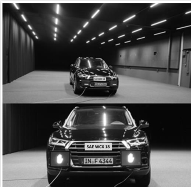
FIGURE 19 Test setup for the evaluation of 1-D and 2-D Signalling functions for autonomous driving.
