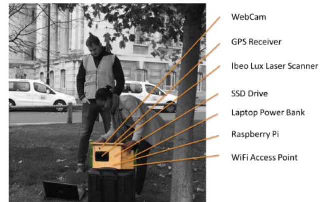
Figure 22: Depiction of the finalized prototype used by Observers in Leeds
