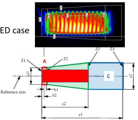
A: contains left end turn of filament B: is covered by filament horizontally C: contains right end turn of filament
