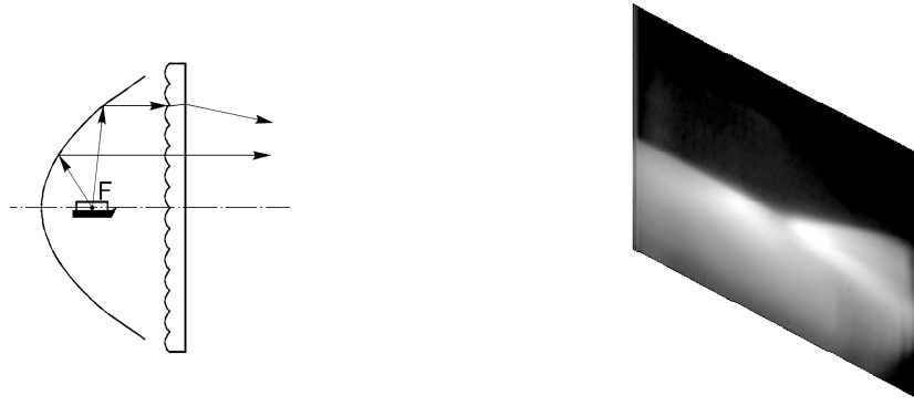
Figure 9. Schematic and beam pattern example of paraboloidal headlamp design with shielded filament. It cause relatively uniform illumination in whole part of screen under cut-off and only some additional light close to needed maximums (50R, 75R)
