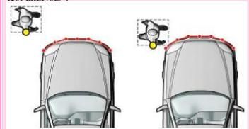
Test setup : need to define a % of vehicle width for both C2C and C2P to characterize impact location when no braking action is applied.
