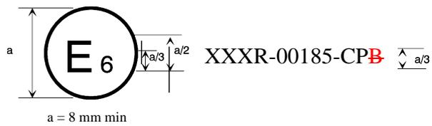
The above approval mark affixed to a vehicle shows that the vehicle type concerned has been approved in Belgium (E 6) with regard to the Advanced Emergency Braking Systems (AEBS) pursuant to Regulation No. [XXX] (marked with C for Car to Car, P for Car to Pedestrian, ~~B for Car to Bicycle~~). The first two digits of the approval number indicate that the approval was granted in accordance with the requirements of Regulation No. [XXX] in its original form.
