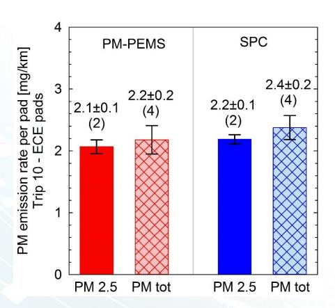
No statistically significant differences could be observed between the SPC and PM-PEMS mass emission rates in the subset of data in which the SPC operated without the dilution tunnel (49 Nlpm sample flowrate).
