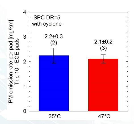
Effect of filter temperature was investigated for ECE pads in limited tests with the SPC operating with its dilution tunnel.
