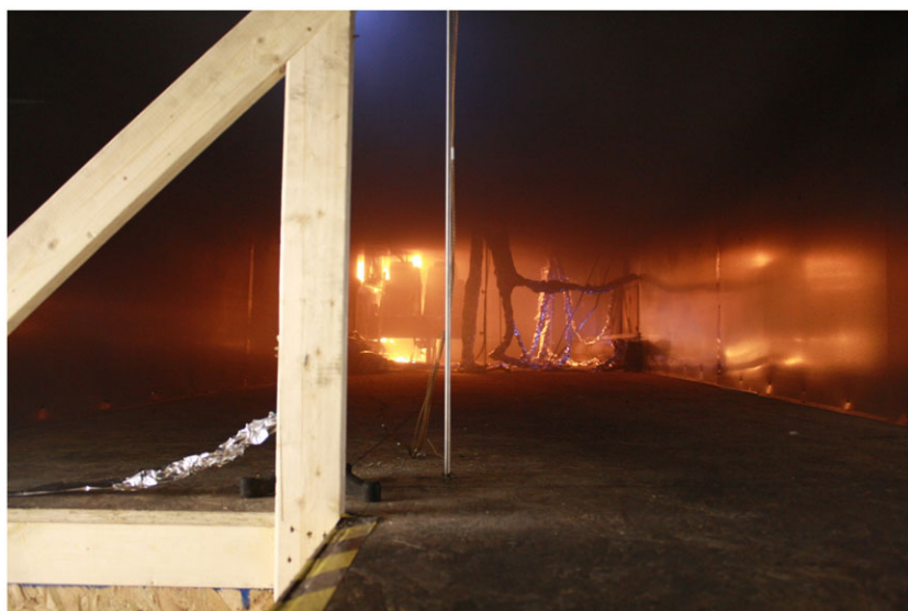
FIGURE 8 Tenability experiment passenger compartment about 15 minutes after burner removal [Colour figure can be viewed at wileyonlinelibrary.com ]
