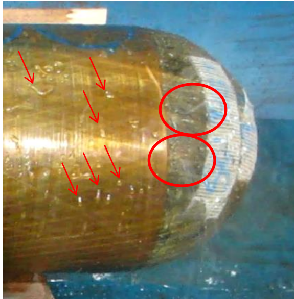
Figure 17. Leakage from dome and sidewall of container 3-E during hot pressure cycling
