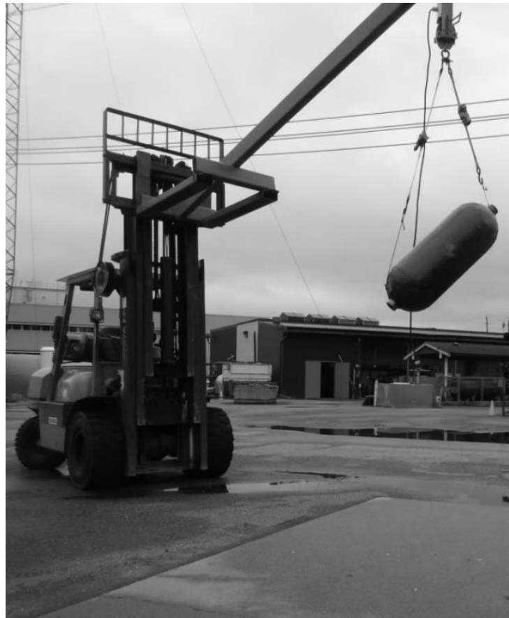
Figure 4: Drop Test Setup
