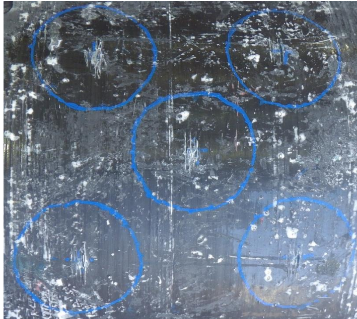
Figure 10. Container 2-E after pendulum impact
