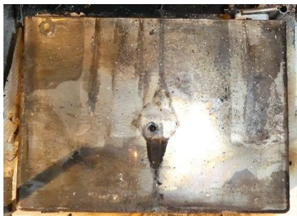
Steel nail, #28, full penetration
