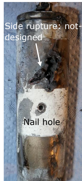
Ceramic nail #7 full penetration
