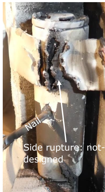
Steel nail #15 full penetration
