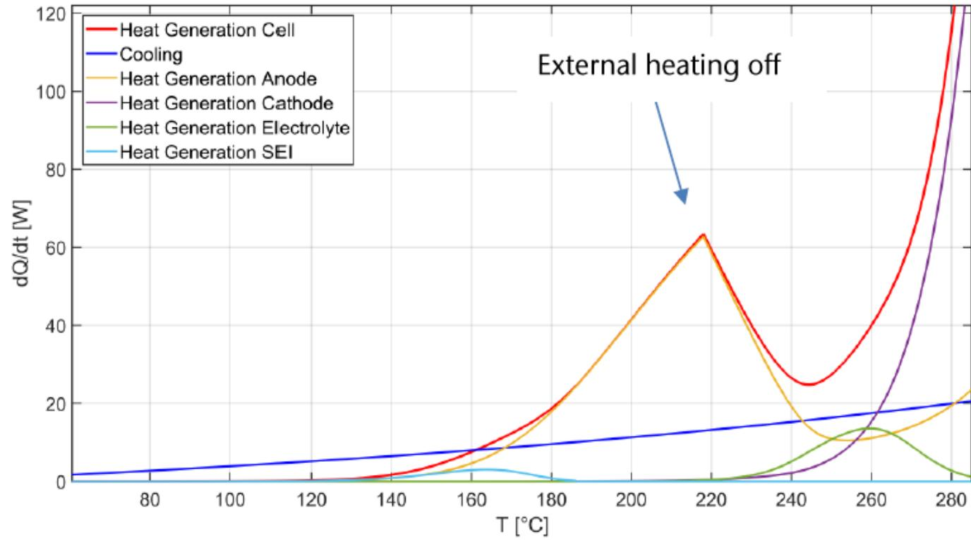
*Simulation results of Thermal Runaway initiated by external heating shown as Semenov Plot.*
