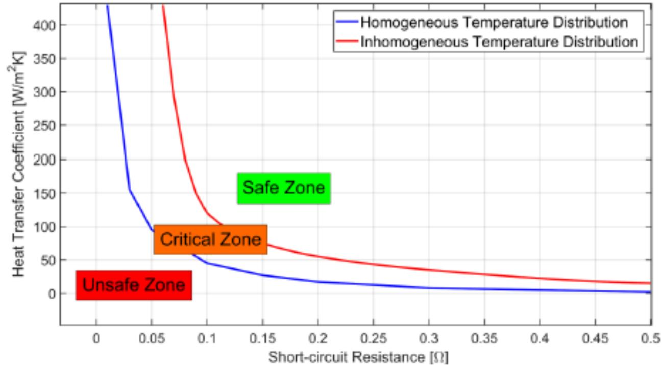
*Analysis of different short-circuit resistances on the effect on the critical heat transfer coefficient in cases of homogeneous and inhomogeneous temperature conduction*
