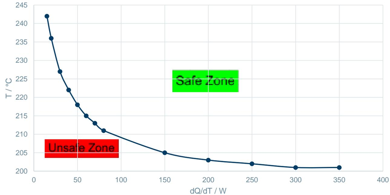
*Critical temperatures at different cooling rates*
