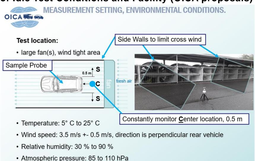
Verify uniformity of wind at two side points, 0.5 m from each side of vehicle
