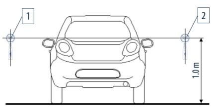
1,2 – anemometers; 3 - weather vane
