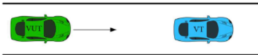
Figure 6.27 Schematic diagram of test scenario that forward vehicle is stationary
