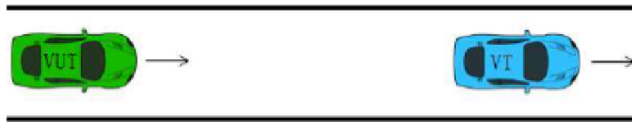
Figure 6.15 Schematic diagram of test scenario of stable vehicle-following driving
