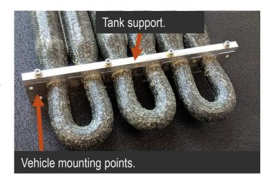
Tank support manufactured and tested with tank. No damage to pressure container during install and service.
