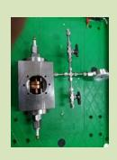
Permeability measurement of O-ring in high-pressure H<sub>2</sub> environment
