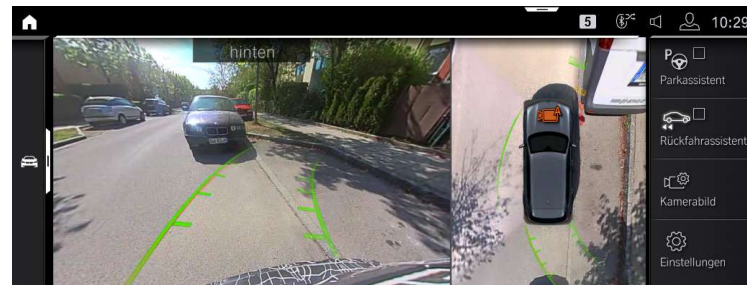
steering wheel turned → Objects are shown which are not visible in fixed rear view!
