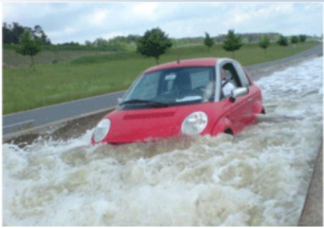
Tests of the Think City (2008) on the movement in the water
