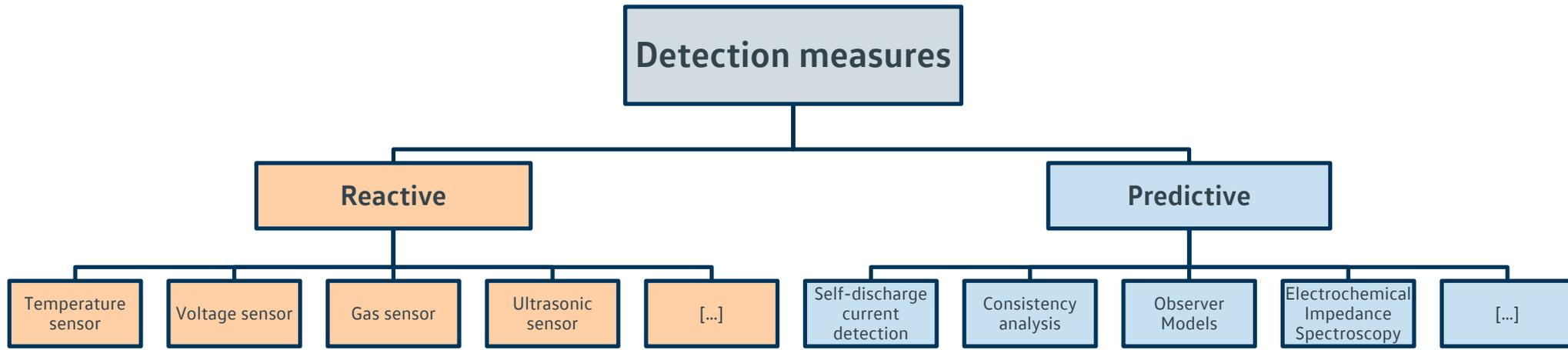
Figure 2 – Classification of detection measures.
