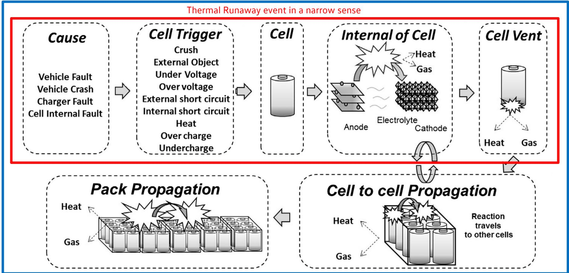
Figure 1 – Observational layer of Thermal Runaway and Thermal Runaway Propagation failure. source: modified, taken from [1]
