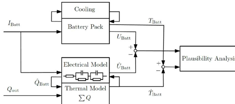
Figure 4 – Illustration of an observer model. source: [3]
