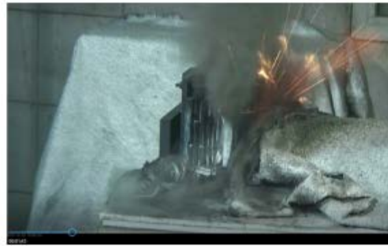
(B) t=105 s - cell #1 in TR; just after grey smoke and sparks appeared
