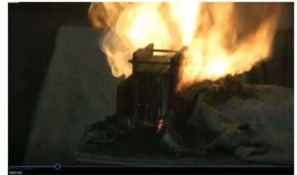
(C) t=113 s - cell #1 in TR; start of fire
