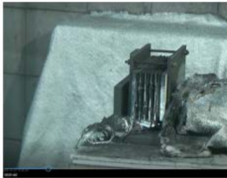
(A) t=100 s - cell #1 in TR; first instance of white smoke appearance (nail penetrates from the right hand side)
