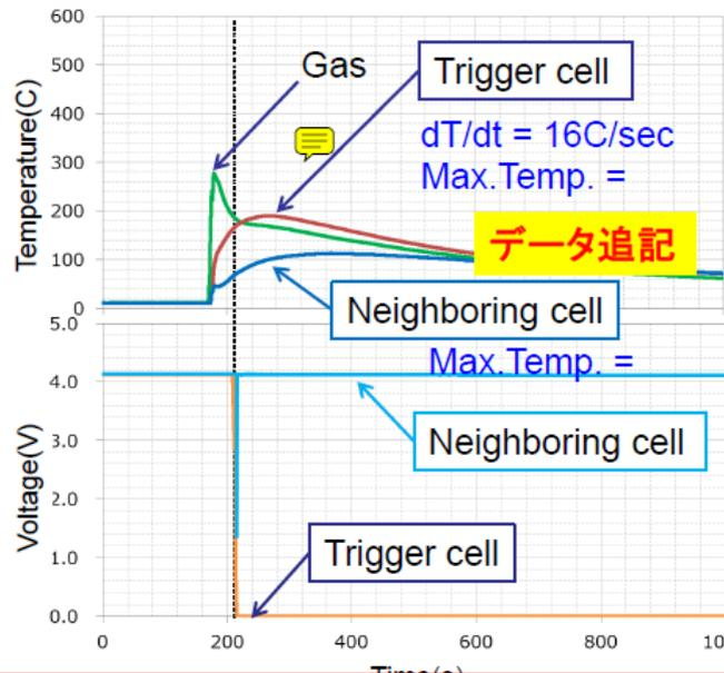
Nail penetration direction needs to be vertical to the electrodes. Nail penetration in a horizontal direction is necessary depending on situations. Depending on the pack or vehicle design, the nail method may not be feasible.
