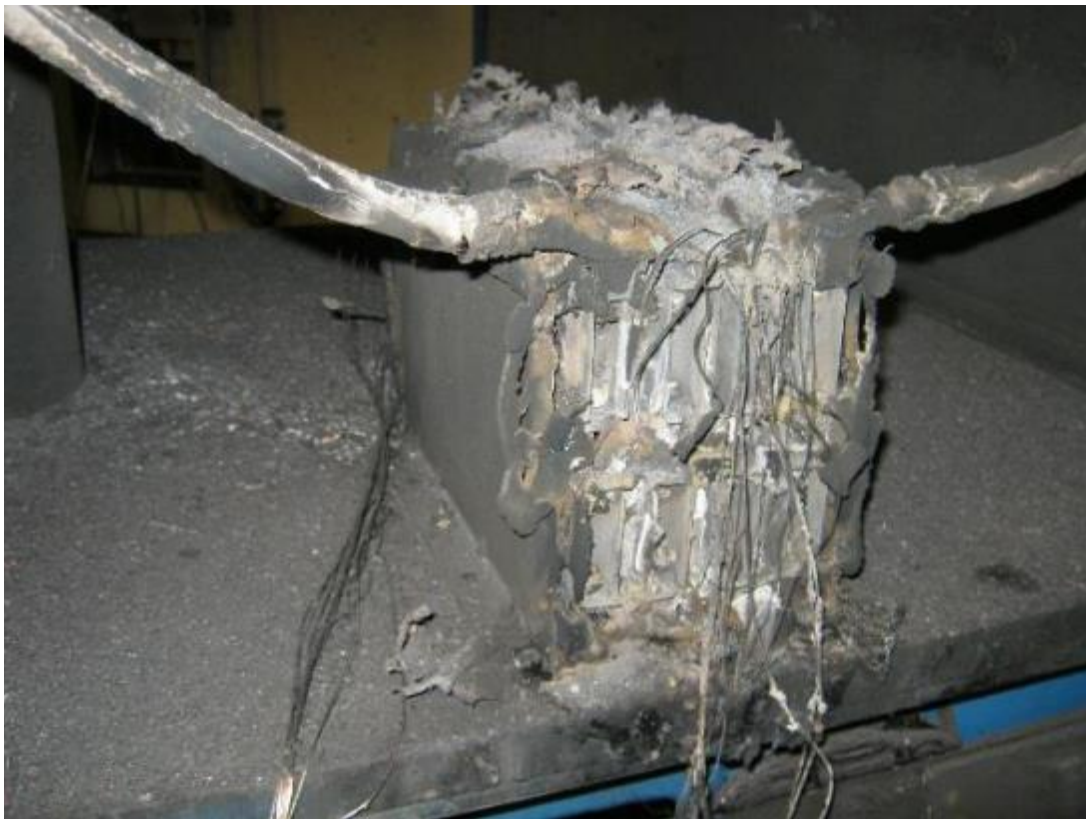
Figure 136 Start/Stop 61A Module Type A Post-Test Fixture (OC027)
