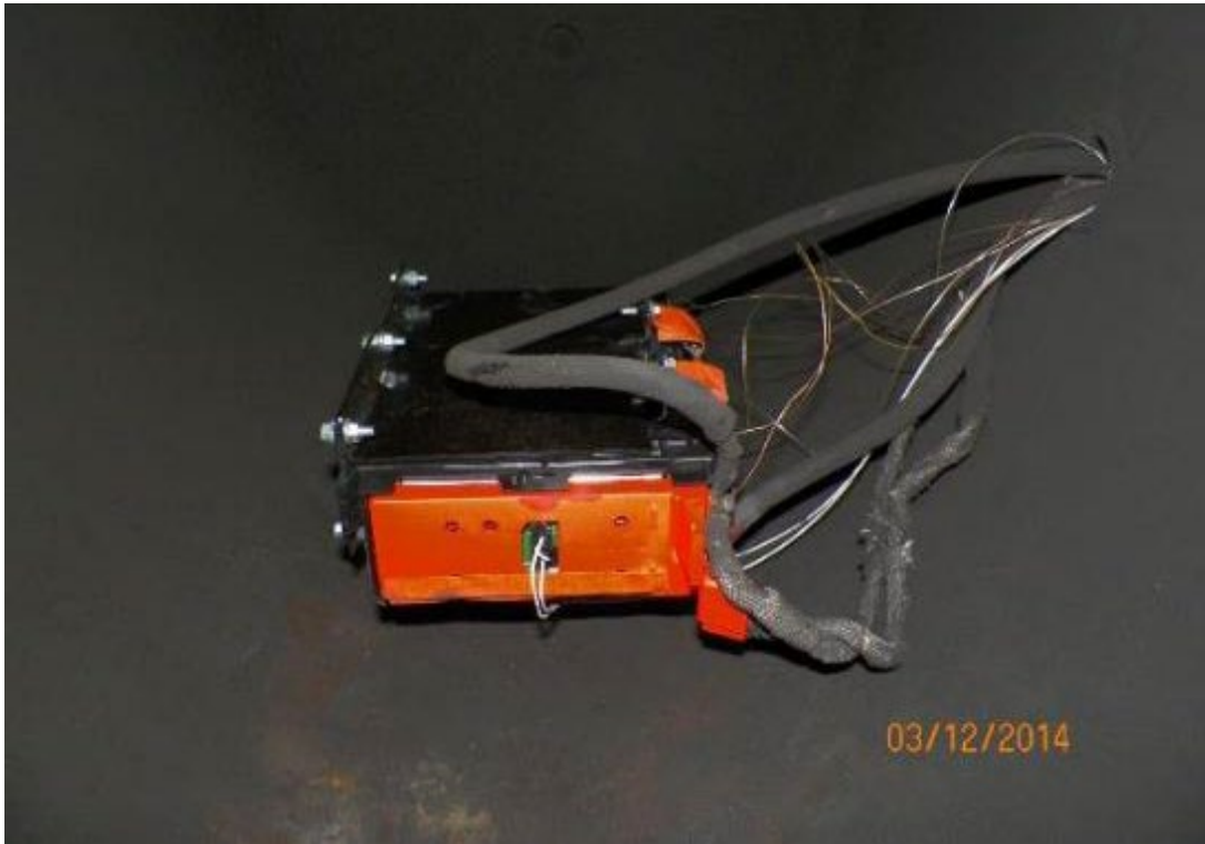
Figure 138 Continuous 155A String Type A Pre-Test Fixture (OCPCA02)
