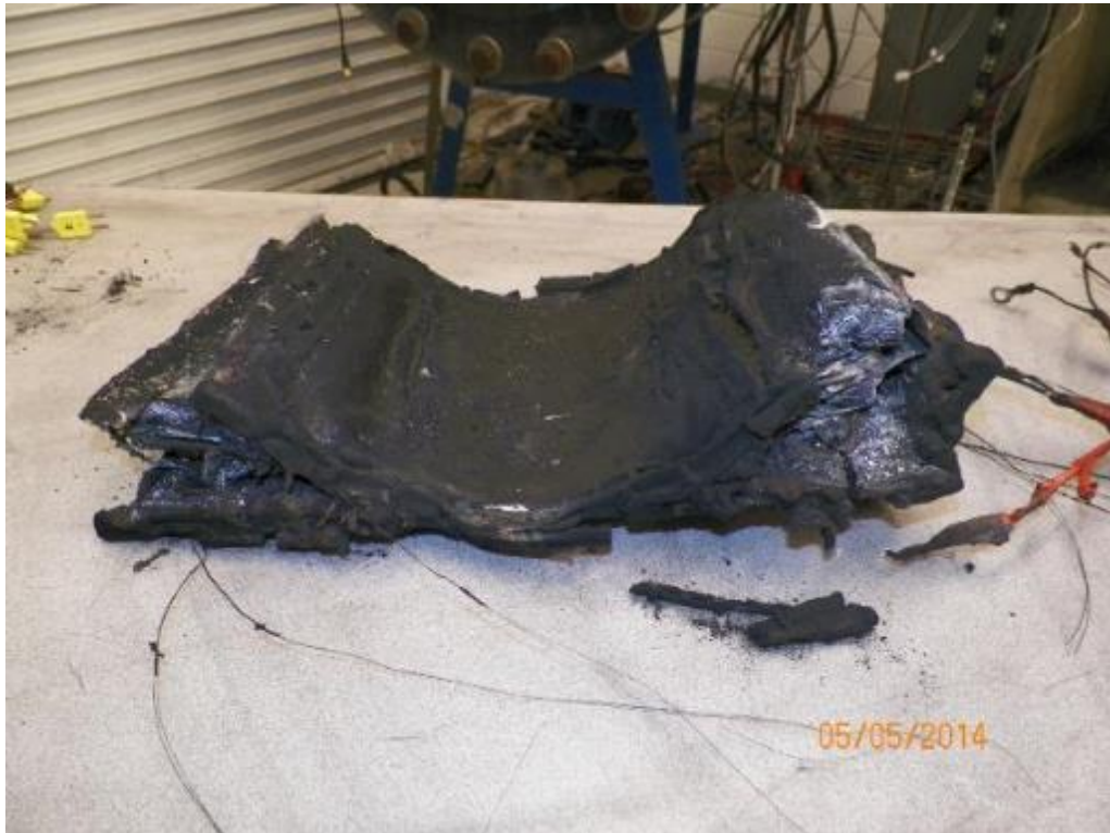
Figure 48 X-Axis Continuous String Type A Post-Test Hardware (CRXCA03)
