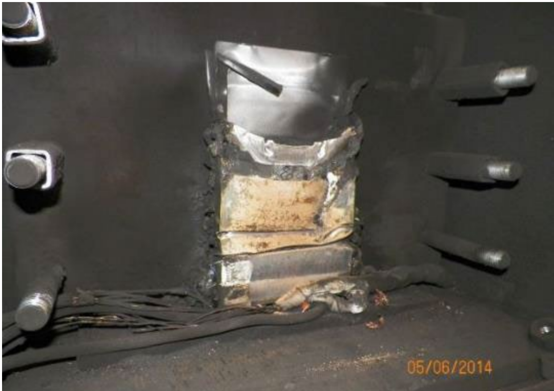
Figure 96 Y-Axis 20-Step String Type B Post-Test Fixture (CRY20SB01)
