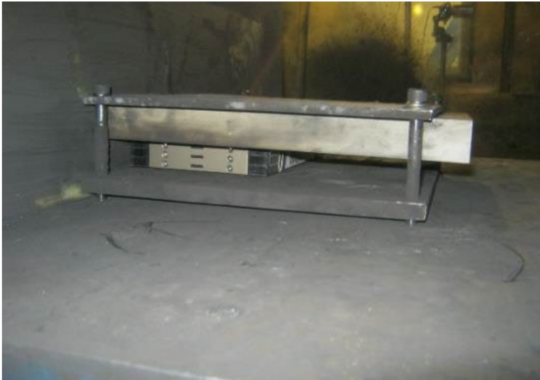
Figure 73 Z-Axis Continuous String Type B Pre-Test Fixture (CR027)
