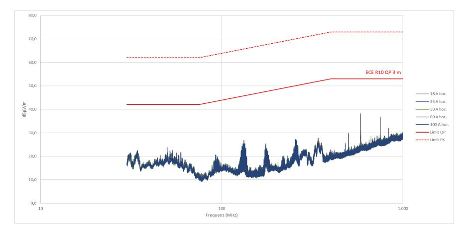
Results of a measurement campain with a BEV (Battery Electrical Vehicle) during a development phase in 3 m distance with Pkdetector. Limits according to ECE R10 (Pk- and QP).
